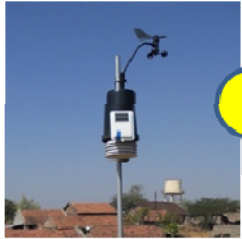
Automated Weather Stations installed in villages
