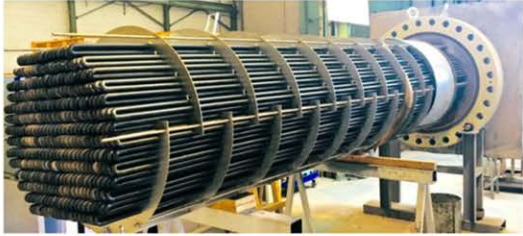
Electric heaters for charging molten salts - fired by PV/wind power
